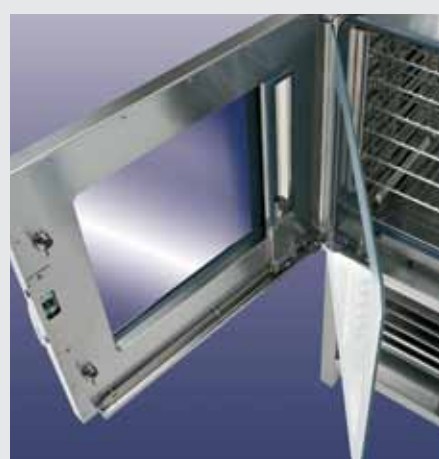
Double tempered glass panels, internal glass panel opens to facilitate air circulation and cleaning operations.
